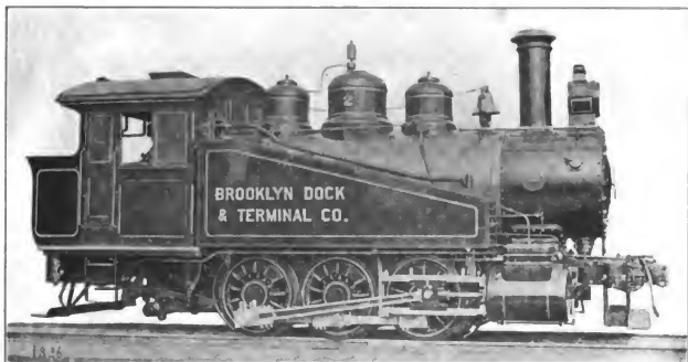
Fig. 13. Six-Wheel (0-6-0) Tank Switching Locomotive. Built by the Baldwin Locomotive Works for the Brooklyn Dock & Terminal Co. Cylinders 19 in. x 24 in..Working Steam Pressure 180 lbs. per sq. in., Total Heating Surface 1,070 sq. ft., Diameter of Drivers 46 in., Weight on Drivers 132,210 lbs., Total Weight 132,210 lbs.
